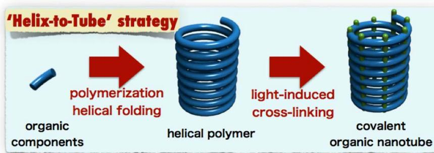
**Figure 3.** New synthetic approach towards covalent ONTs through longitudinal cross-linking between helical pitches in helical polymers.
