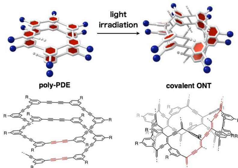
**Figure 5.** Synthesis of a covalent ONT by photochemical cross-linking between longitudinal aligned 1,3-butadiyne moieties (red lines).
