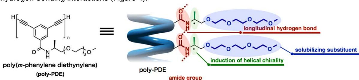
**Figure 4.** Molecular design for helical poly-PDE bearing chiral amide side chains.
