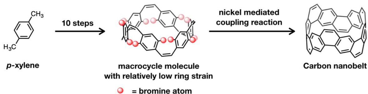
Figure 3. Synthetic approach towards the carbon nanobelt from p -xylene in 11 steps.
