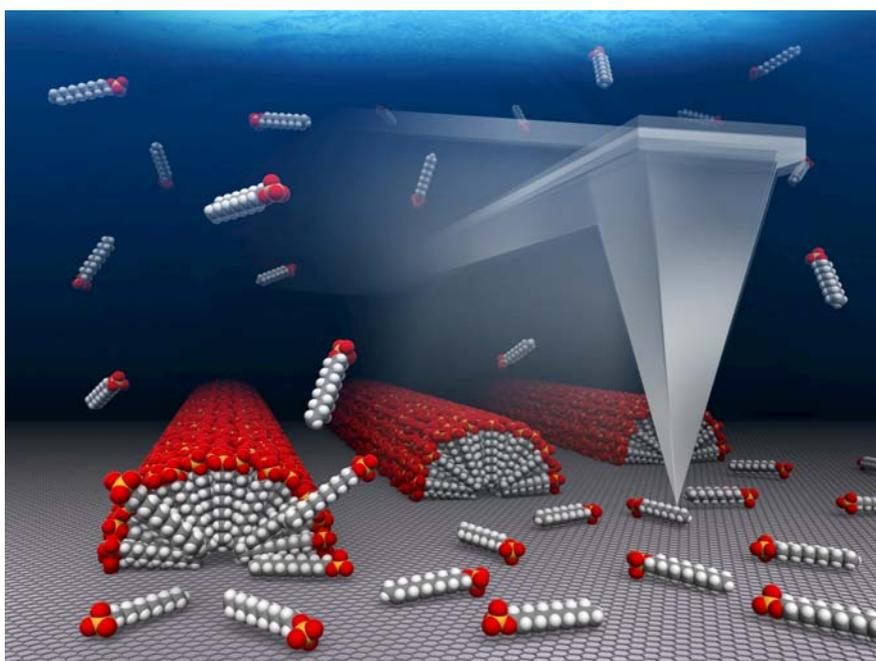
Molecular assemblies on graphene grow in perfect orientation by atomic force microscopy (AFM) tip scanning. The gray plane on the bottom represents the graphene surface. The stick-like particles consisting of red, white, yellow and gray colored balls represent surfactant (sodium dodecyl sulfate (SDS)) molecules. The gray colored reverse pyramid-like structure represents the probe tip of AFM.
