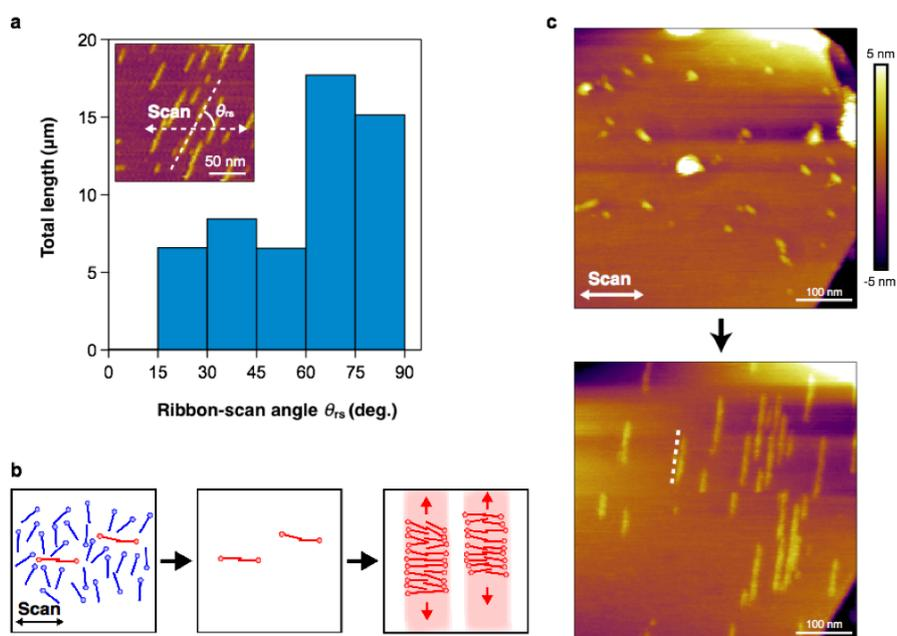
**Figure 3.** (a) Relationship of the total length of the SDS ribbons and the ribbon-scan angle ( $\theta_{rs}$ ) ( $\theta_{rs}$  is defined as the relative angle between the ribbon longitudinal axis and the scan direction as shown in insert figure), (b) Schematic illustration of the mechanism of selective removal of SDS molecules followed by the ribbon growth process, (c) Unidirectional formation of the SDS ribbons from random orientations.
