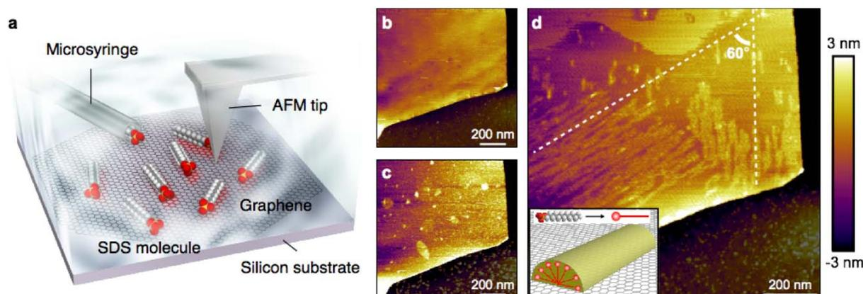
**Figure 2.** (a) Schematic diagram of the experimental setup, (b) AFM height image on the graphene surface in water without SDS molecules, (c) 1 hour after the SDS solution injection, and (d) after 15 minutes of intense AFM scanning
