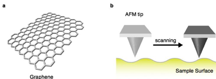
**Figure 1.** (a) Structure of a graphene molecule. Benzene units are fused together in a sheet. (b) Schematic diagram of atomic force microscopy (AFM) measurement.
