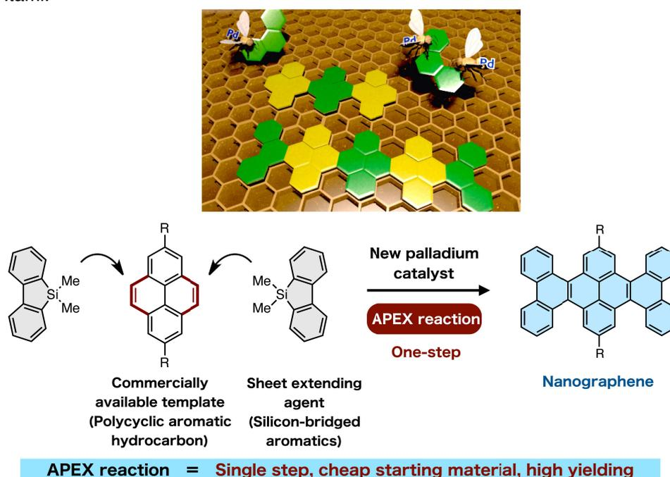
Figure 1. A single-step APEX reaction to synthesize uniform nanographenes. Selective annulation at the 'K-region' leads to direction-controlled synthesis of nanographenes in high yield.
