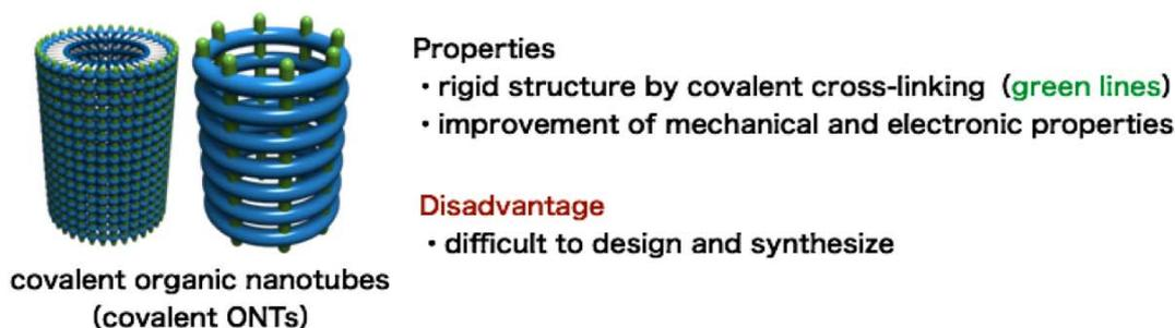
Figure 2. Covalent ONTs derived from non-covalent ONTs by cross-linking, their properties and disadvantages.
